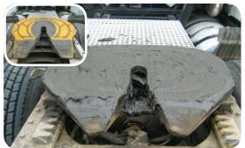
A well-lubricated fifth wheel enhances vehicle performance. "Fifth wheel steer" is minimized by continuous lubrication of the fifth wheel.
