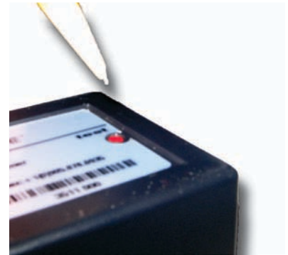
Illustration 15. Location and method to push test button on timer.
