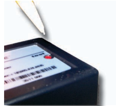
Illustration 28. Location and method to push test button on timer.
