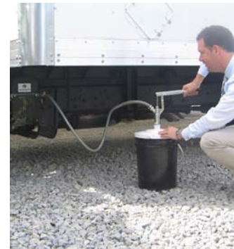
Illustration 36. Fill the reservoir until maximum level.
