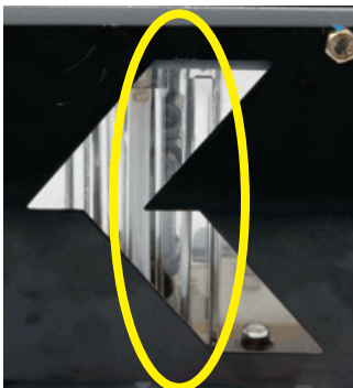
Illustration 37. Overflow tube in front center of the pump.
