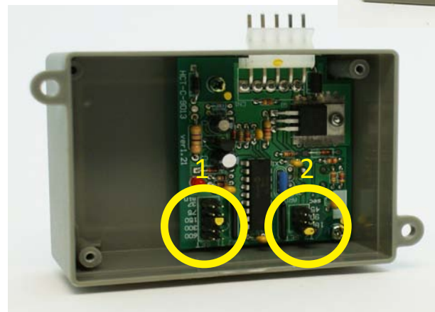
Illustration 27. Jumper-peg locations for timer pause and working phase adjustments.
