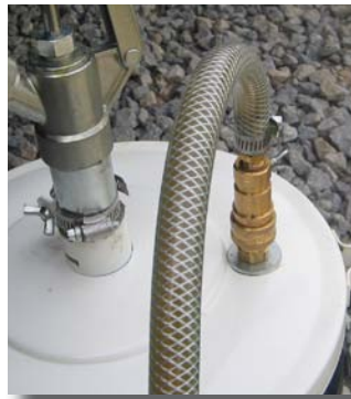
Illustration 35. Circulate grease to remove air pockets.
