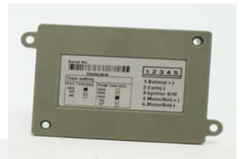
Illustration 26. Jumper peg wiring chart located on the bottom of the LCT timer.
