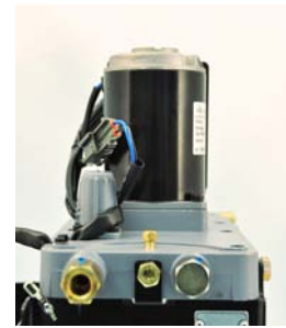
Illustration 11. Side view of pump electric motor. Main supply port can be seen in the lower left hand corner of the photo.
