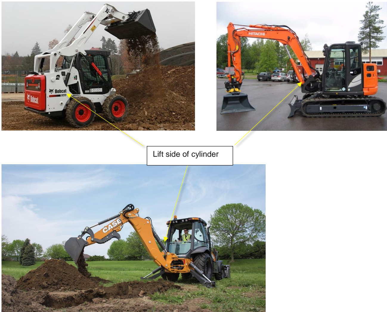
Figure 19 Lift side of cylinder on various equipment examples
