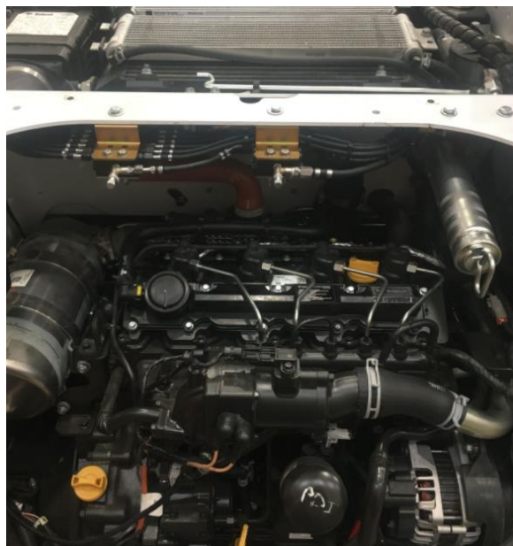
Figure 15 Pump Installed in Skid Steer Engine Compartment
