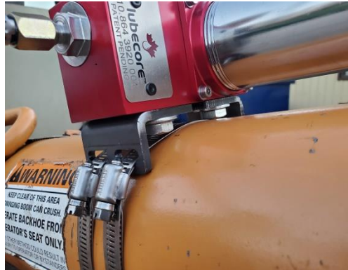
Figure 10 Band Clamps with Mounting Brackets on Cylinder
