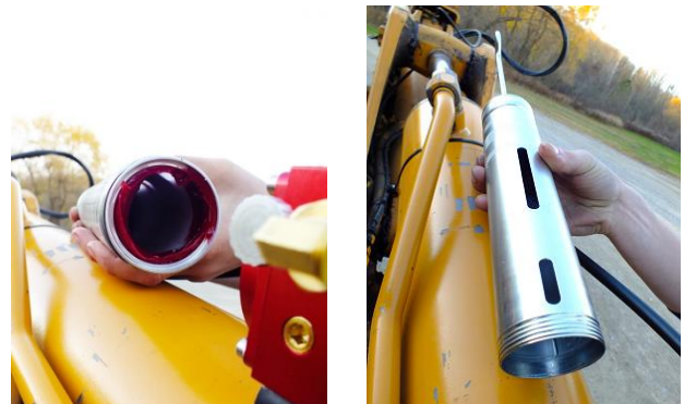
Figure 29 Removing empty grease tube
