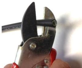
The Korilla hose can be cut with a knife, pruning scissors or Synflex cutters
