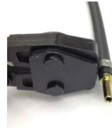
The stainless steel crimp style clamps can be crimped with standard tools.
