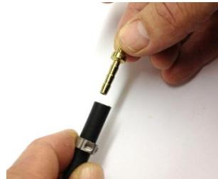
The barbed inserts are inserted either by hand or using a Lubecore Insertion tool depending on which insert is being used
