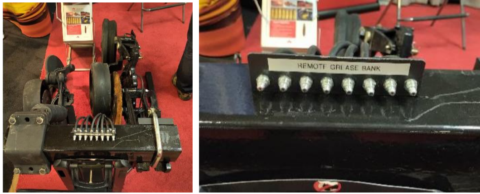
Figure 3 Grease Bank Installed on a
