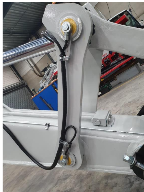
Figure 2: Installed Heavy-duty Banjos
