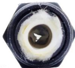
Figure 14: Improper Installation restricted grease path
