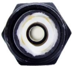
Figure 13: Proper Installation unrestricted grease path
