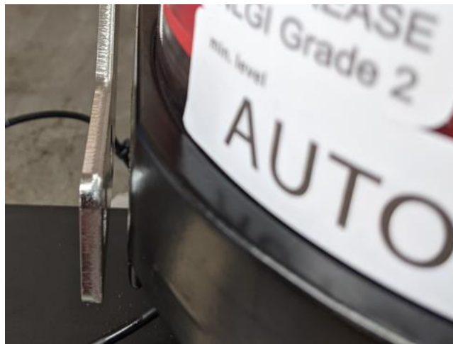
Figure 1: The one-piece mounting brackets are designed to have clearance between the bracket and the pump
