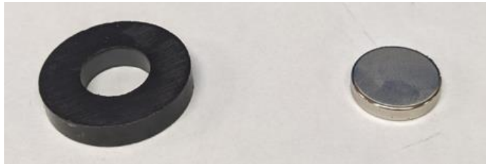
Figure 3: Lubecore's standard timer magnet (left) and temporary alternative (right)
