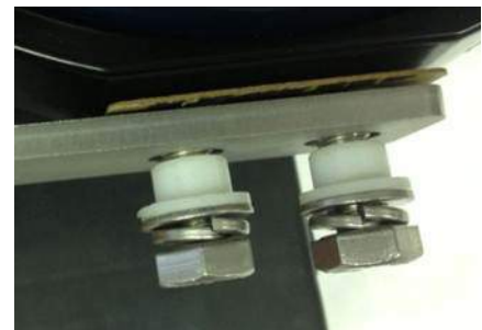
Illustration 18. Pump Bracket Mounting Hardware Assembly Order. (Pre-tightening)
