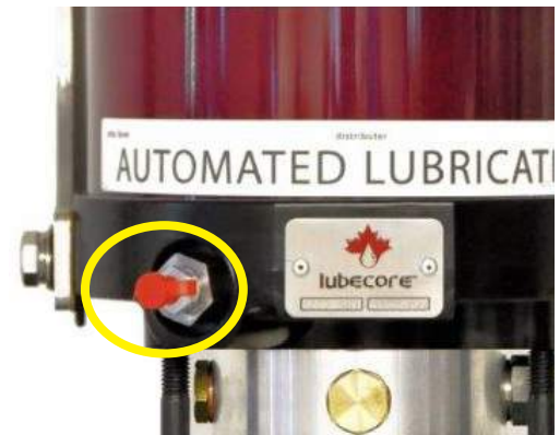
Illustration 35. Male Filler Coupling with Dust Cap. Either a Regular Grease Zerk for EP2 Grease or a Male Quick Disconnect for EP0 Grease.
