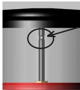
Illustration 36. Overflow Opening in the Center Guide Rod.
