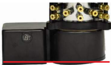
Illustration 13. Sloped Housing Prevents Moisture Build Up.
