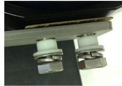
Illustration 19. Pump Bracket Mounting Hardware Assembly Order. (Pre-tightening)
