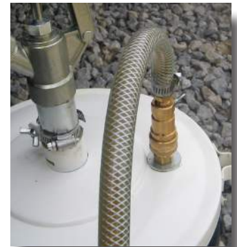
Illustration 34. Circulate Grease to Remove Air Pockets.
