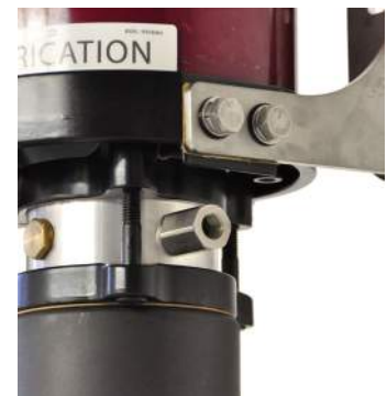
Illustration 27. Pump with Single Metering Element Installed.
