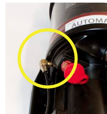
Illustration 12. Left Side view of Pneumatic Pump with Overflow circled.
