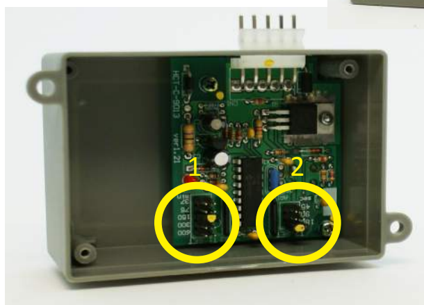
Illustration 24. Jumper-Peg Locations for Timer Pause and Working Phase Adjustments.
