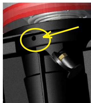
Illustration 56. Overflow Opening on the Left Side of the Pump.
