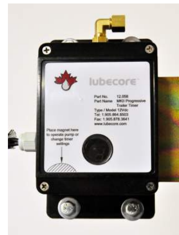
Illustration 36. Lubecore 12 VDC Electrically Operated Progressive Trailer Timer for ALS (12.058)
