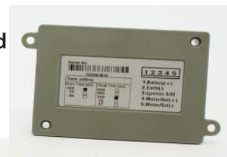
Illustration 23. Jumper Peg Wiring Chart Located on the Bottom of the LCT Timer.
