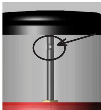
Illustration 57. Overflow Opening in the Center Guide Rod.
