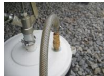
Figure 4852 Pail hose quick disconnect returned to mating lid fitting
