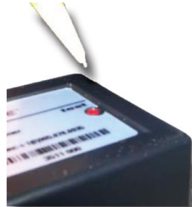
Figure 2527 Location and Method to Push Test Button on Timer.
