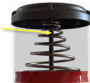
Figure 1044 Cross section of the reservoir follower plate and guide rod with over flow openings highlighted
