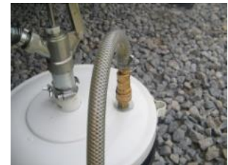
Figure 4347 Step 2: Circulating Grease
