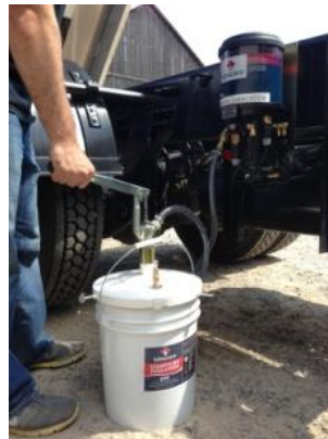
Figure 4448 Steps 3 and 4: Filling the reservoir
