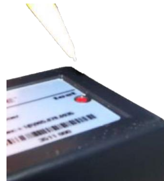
Figure 1547 Location and Method to push Test Button on Timer.
