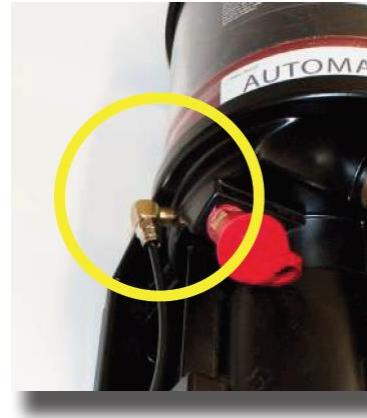
Figure 1214 Left side view of pneumatic pump with overflow circled
