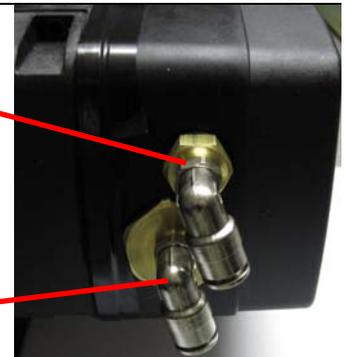
2. The Air Signal line is to be plugged or, disconnected from the trailer system. The fitting in the air signal position is to be removed and replaced with a plug. Remove the elbow fitting and brass body of the air supply position.
