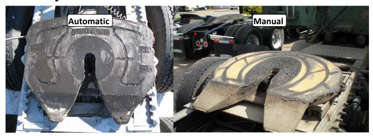
Pictured above are two fifth wheels. Manual service to the fifth wheel on the right has not been able to provide the appropriate grease level. Automated lubrication has been applied to the plate on the left, and grease levels have been maintained while the truck was hooked up to a trailer.
