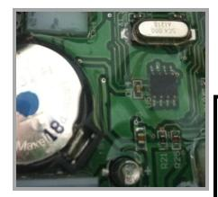
All Mk2 trailer timers are now epoxied with a transparent, mildew, corrosion, acid and heat resistant compound that encapsulate all the electronics mounted on the printed circuit board. Effectively encasing everything in a polymer that sheds condensation and dirt like water off a ducks back, and acts as a shock absorber alleviating any possibility of damage from vibration.
