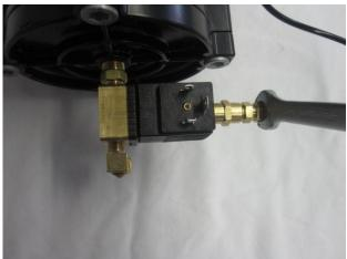
Remove the airline connection from the air source on the equipment using a 9/16" wrench.
