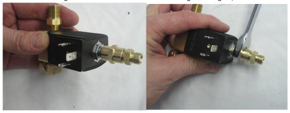
Install the solenoid assembly back on the bottom of the pump using a 9/16" wrench remembering to face the solenoid in the same direction as was when you took it off so that all your connections will line up.
