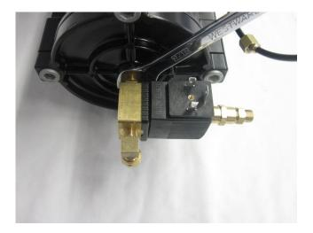
Connect the airlines and electrical wire. Test to ensure solenoid is functioning properly.
