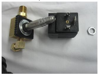
Remove the black plastic cover from the assembly as shown below. This will expose the four socket head cap screws that hold the solenoid spring assembly in place.
