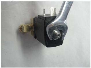
Install the brass straight connector back on the solenoid and tighten using a 9/16" wrench.
