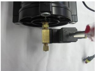
Remove the short piece of empty single line from the side of the solenoid using a 12 mm wrench.
