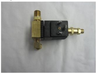
First you need to remove the brass straight connector from the head of the solenoid using a 9/16" wrench.
