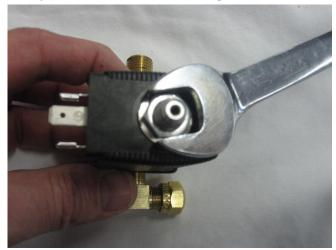
Remove the nut and you will be able to slide the black assembly off of the solenoid spine
