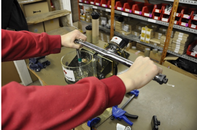
Torque bolts to 7.5 in/lbs
