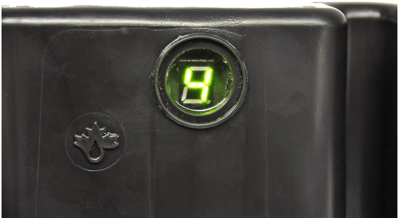
LED Display showing timer program code.
