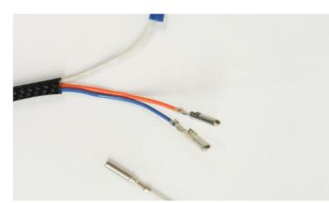
**5.** Connect wiring to Lubecore timer. Orange wire attaches to #8 on timer. Blue wire attaches to #11 on timer. White attaches to 6pin Deutsch Common Ground on 13.047 timer harness. (Further instructions available on document 75.001).
