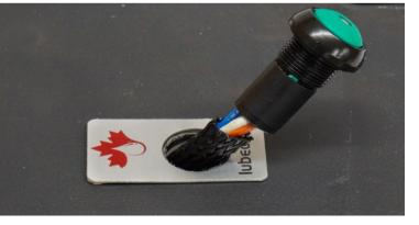
**4.** Pull Lubecore system Smart Switch through the hole created. Take 1/2 inch nut and thread onto the back of the test light, do not over tighten.
