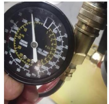
Vacuum created through quick disconnect filler - Undesirable
