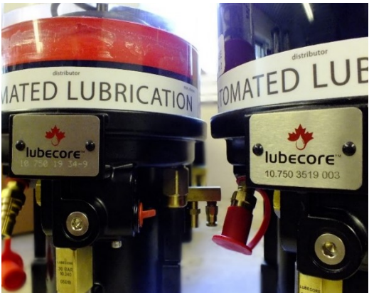
Pump Serial Plate Marking: Dot marking vs. Laser
