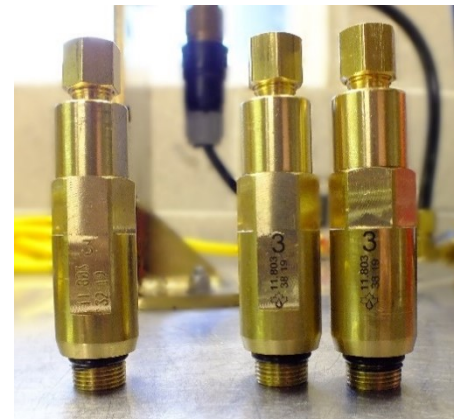
Brass Super Injector Dot Marking vs. Laser
