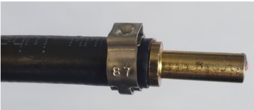
Figure 4: Location of clamp relative to the end of the Korilla lining.
