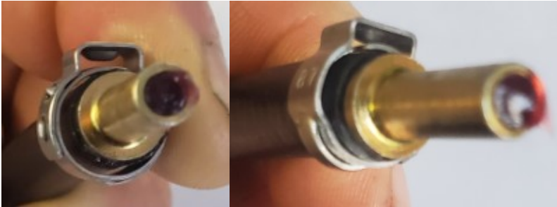
Figure 3: Left to Right: Improper Loose Fit of 20.232, Proper Close Fit of 20.239
