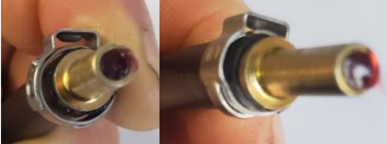
Figure 4: Left to Right: Improper Loose Fit of 20.232, Proper Close Fit of 20.239
